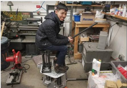
**Hagrid's Wild Ride** was a haptic Virtual Reality flight simulator with a Harry Potter Quidditch theme. We designed a novel spring-based haptic rig that does not rely on expensive actuators to create a realistic and immersive flight experience.
